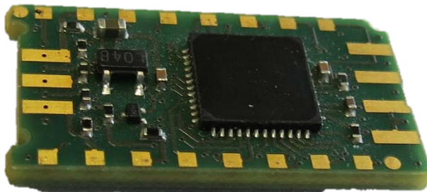
AirChip3000 installed on its small companion PCB
