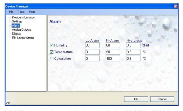
**Note**: This function has no effect on the HF6 analog outputs and applies only to the HF6 optional display (an alarm symbol appears) and to the HF6 digital communication with a PC via service connector.
