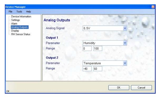
Analog signal: the type of signal for both analog outputs of the HF63 (3-wire circuit type) can be configured with HW4 as shown below:
