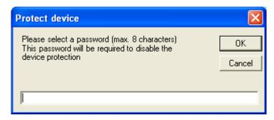
Click on the Device Manager OK button to write the new protection settings to the HF6.
