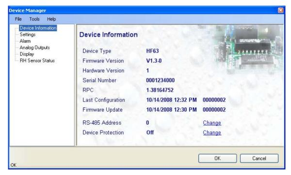
The different sub-forms that are available within the Device Manager form are listed in a tree located on the left pane of the form. The number of sub-forms depends on the HF6 model (Device Type). To select a sub-form, click on it with the left mouse button.
