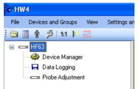
Click with the left mouse button on Device Manager to open this module. HW4 opens the Device Manager form.
