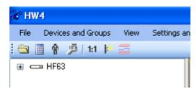
When HW4 detects a HF6 transmitter, the device appears as an icon in the left pane of the HW4 main screen. Click on the + sign to the left of the HF6 icon to display a list of the available functional modules.
