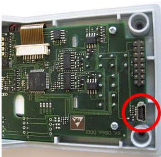
Figure 19: Location of the service port on the top side of the circuit board
