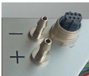
Figure 7: Differential pressure connections and E2 socket on the bottom side of the PF4
