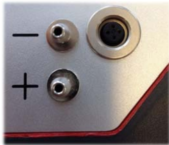
Figure 10: Pt100 and differential pressure connection on the bottom side of the PF4
