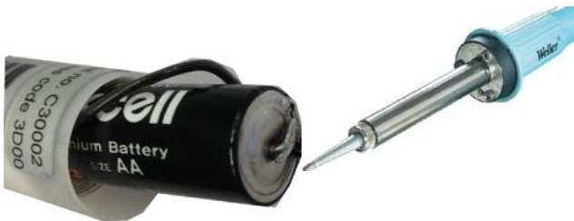
Figure 13: Unsoldering the battery
