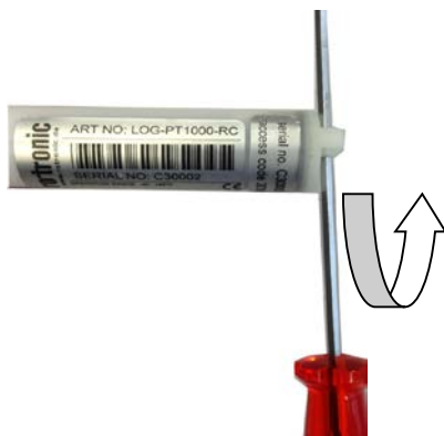
Figure 11: Unscrew cover with screwdriver
