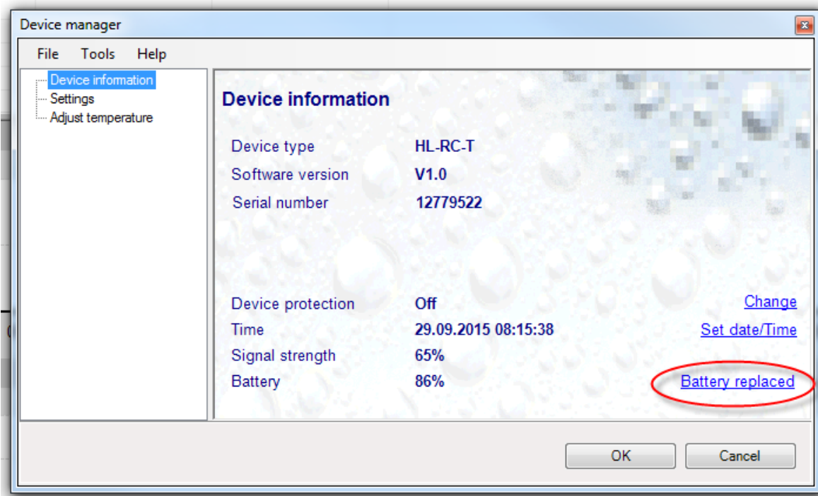
Figure 16: Setting the time after a battery change
