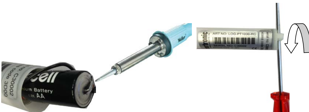
Figure 15: Soldering the solder connections and subsequently screwing on the cover
