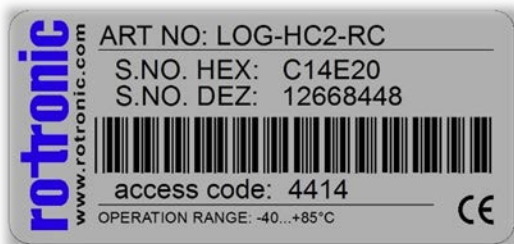
Figure 10: Label with access code (4414) to disable/enable the logger
