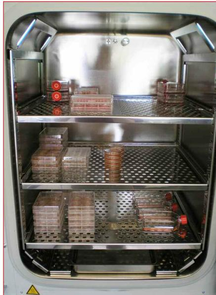
*The interior of a CO<sub>2</sub> incubator.*
