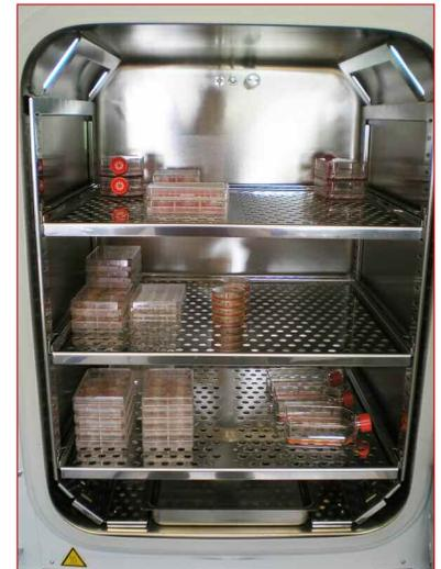
Inside a cell culture incubator. . . the interior of a CO<sub>2</sub> incubator.
