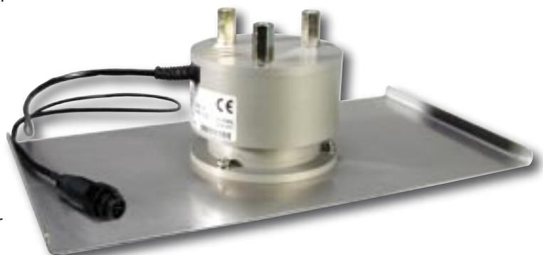
The BFC-DIO probe is used in combination with a HygroFlex transmitter. With active extensions cables, probes can be placed up to 200 m from the transmitter. It is possible to connect up to 2 probes simultaneously to the HygroFlex-3 transmitter, and up to 32 transmitters can be networked using the RS485 interface, allowing multiple measurement points to be monitored using a single PC.
