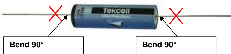
Figure 14: Shortening and bending the connections
