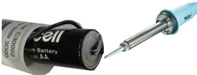
Figure 13: Unsoldering the battery
