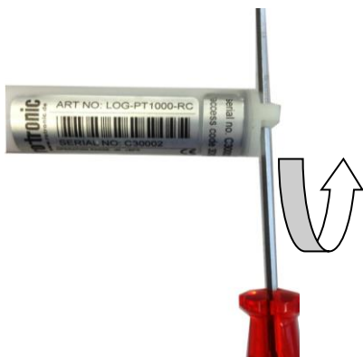
Figure 11: Unscrew cover with screwdriver
