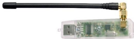
Figure 7: USB dongle for 433.92 MHz (Europe) or 915 MHz (USA); can manage up to 100 terminal devices
