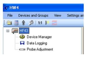
To select the Device Manager module, click on it with the left mouse button. HW4 opens the Device Manager form.
