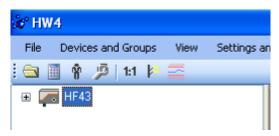
When HW4 has detected a HF4 transmitter, the HF4 appears as an icon in the left pane of the HW4 main screen. Click on the + sign to the left of the HF4 icon to display a list of the available functional modules.
