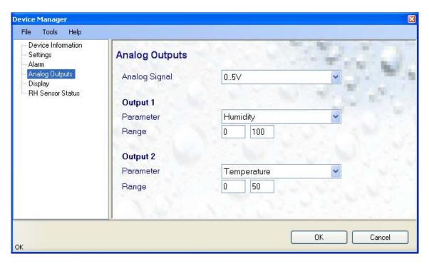
Analog signal: the type of signal for both analog outputs of the HF43 (3-wire circuit type) can be configured with HW4 as shown below:
