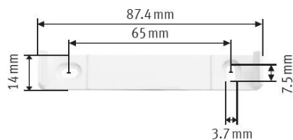
Figure 2: Dimensions of the housing
