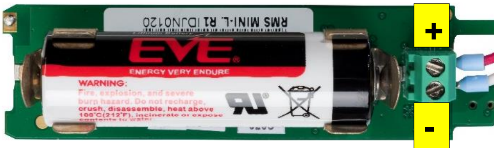
Abbildung 4: Minus pol direction to the button
