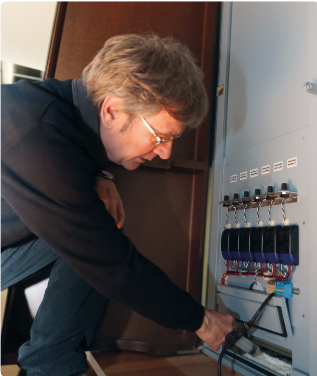
Christian Cevey tops up water in the glass cabinet directly to adjust the relative air humidity.
