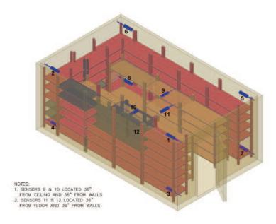
Sensors should be placed in typically known reduced air flow locations. This diagram may not be representative of actual chamber shelves, racks, or cages used to store samples. The table below describes actual sensor placement locations.
