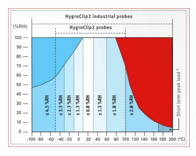
Relative humidity instrument accuracy varies at different temperatures.
