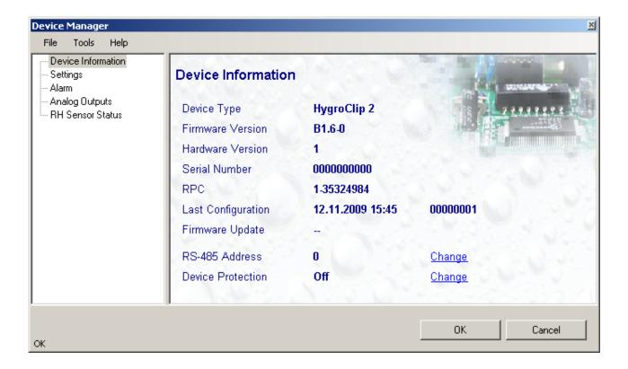
Click on the blue link next to the RS-485 address to open the following form and change the address:
