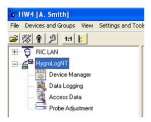
When HW4 has discovered a HygroLog NT or any other type of legacy instrument, the device appears in the left pane of the HW4 main screen. Expanding the device displays a list of the available device functions.
