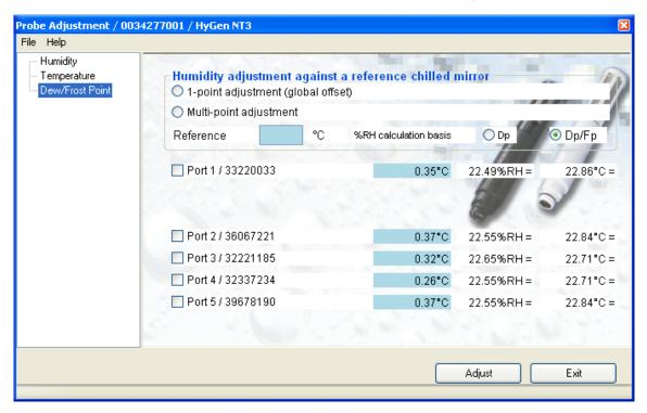
The form displays the dew/frost point, humidity and temperature data from each probe connected to the instrument. The dew or frost point data is shown on a blue background indicating that this parameter will be adjusted.
