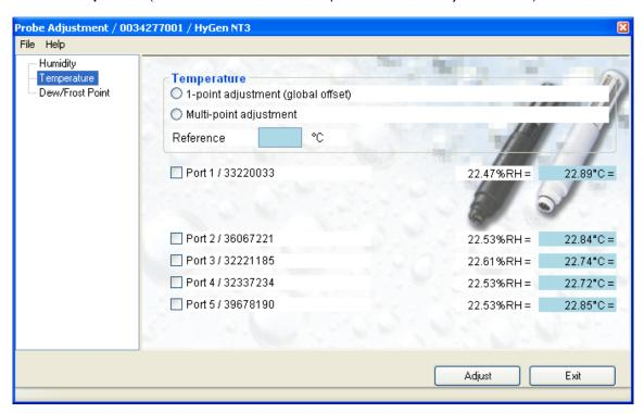
The form displays the humidity and temperature data from each probe connected to the instrument. The temperature data is shown on a blue background indicating that this parameter will be adjusted.
