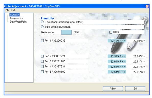
The form displays the humidity and temperature data from each probe connected to the instrument. The relative humidity data is shown on a blue background indicating that this parameter will be adjusted.
