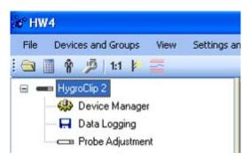
To select the Probe Adjustment module, click on it with the left mouse button. HW4 opens the Probe Adjustment form.
