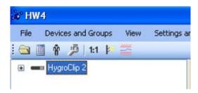
When HW4 has detected a HC2 probe or other AirChip 3000 device, an icon appears in the left pane of the HW4 main screen (HygroClip 2 probe in this example). Click on the + sign to the left of the icon to display a list of the available functional modules.
