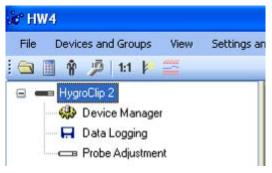
The Data Logging module is used to program the HC2 probe to record data and to read recorded data from the probe.
