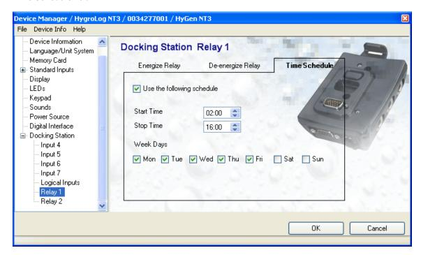
Use this tab to define when the relay is used to monitor the alarm conditions selected in the Energize Relay Tab.
