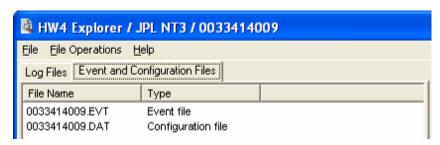
A file with the extension .EVT and one with the extension .DAT are always present in the memory card. These files cannot be deleted with HW4.
