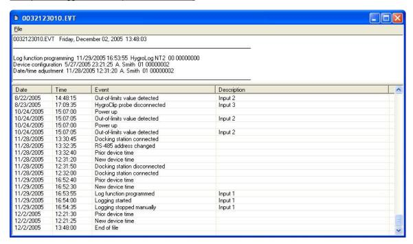
The HygroLog NT keeps internally track of the last 170 operations, events and configuration changes in its internal EEPROM memory as well as in the .EVT file located on the memory card.
