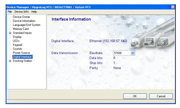
This form is used to select the RS-232 / RS-485 baud rate between 57600 (factory default) and 19200. Other data cannot be changed from within the form. Generally, leave the baud rate at 57600. Select 19200 when you plan on connecting a mix of HygroLog NT and other devices such as the HygroFlex transmitter to an RS-485 multi-drop.
