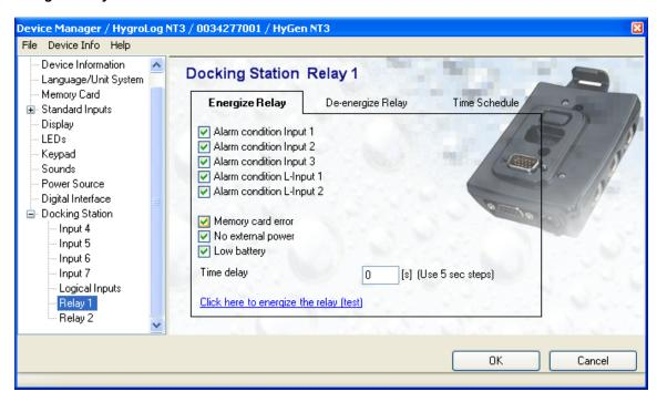
Use this tab to select from the list one or several alarm conditions that will cause the relay to be energized. Alarm conditions for probe inputs 1 to 3 and logical inputs 1 and 2 are defined in Device Manager under "Input" and "Logical Inputs". To associate an alarm condition with the relay, click on the corresponding check box. A check mark symbol appears. Click again on the box to remove the check mark and deselect the condition.
