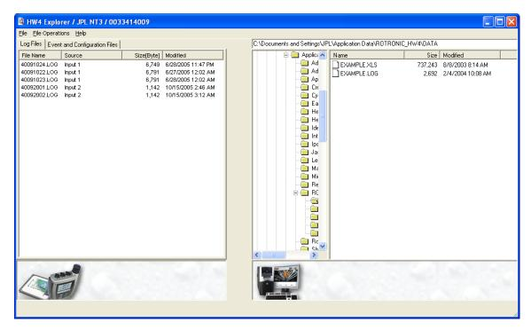
• Left Pane: the left pane of the HW4 Explorer form provides a list of the files currently present in the memory card of the HygroLog NT. Select the Log file tab to view log files. Select the Events and system data tab to view the logger event file (extension .EVT) and the logger configuration file (extension .DAT).
