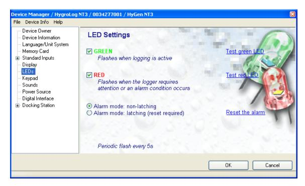
Each of the two LEDs of the HygroLog NT can be enabled or disabled. Each LED can be tested by clicking on the corresponding underlined link. During the test, the LED stays on for a few seconds.
