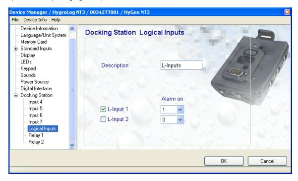
Enter a global description for the two logical inputs and define any condition that you may want to monitor for the purpose of providing an alarm.
