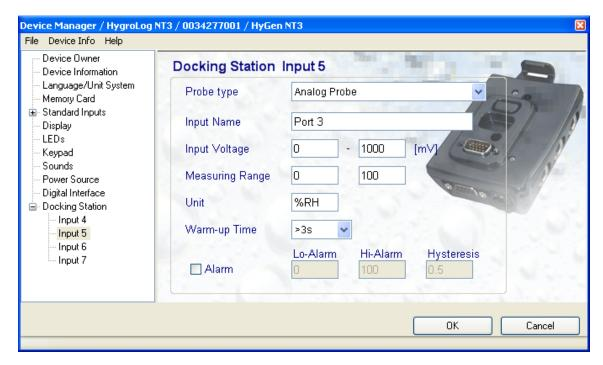
Enter a description for the probe. Specify the range of the input voltage, the measuring range of the probe, the engineering unit of the parameter measured by the probe, the time required by the probe to warm-up, and any alarm values that you may want to use.
