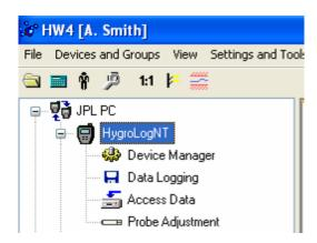
When HW4 has detected a HygroLog NT, the device appears in the left pane of the HW4 main screen. Expanding the device displays a list of the available device functions.
