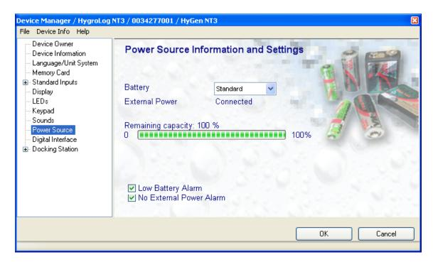
• Type of internal power source: click on the arrow located to the right of the list box and choose between battery and accumulator (rechargeable battery). Note that trying to recharge a regular battery is potentially dangerous and may damage the instrument.
