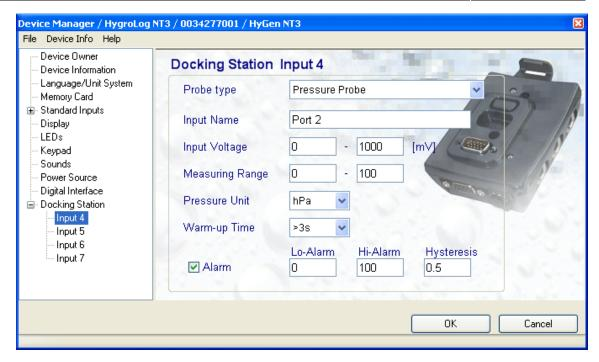
Enter a description for the probe. Specify the range of the input voltage, the measuring range of the probe, the engineering unit used for pressure, the time required by the probe to warm-up, and any alarm values that you may want to use.
