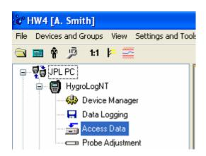
When HW4 has discovered a HygroLog NT, the device appears in the left pane of the HW4 main screen. Expanding the device displays a list of the available device functions.
