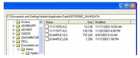
Any file present in the memory card can be opened, copied or moved to the computer, or deleted from the memory card. The logger event and logger configuration files are also present in the internal EEPROM of the HygroLog NT. If not present, these two files will be automatically written to the memory card by the logger. Files that are on the computer can be either opened or deleted. These files cannot be copied or moved to the memory card.
