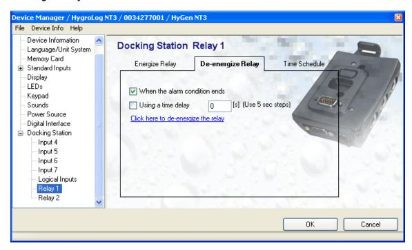
Use this tab to define how the relay behaves when the alarm condition(s) ends.
