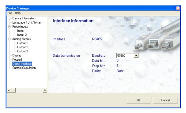
This form is used to select the RS-232 / RS-485 baud rate between 57600 and 19200. Other data cannot be changed from within the form. Generally, use a baud rate of 19200 when you plan on connecting more than 2 or 3 HygroFlex transmitters and similar devices to an RS-485 multi-drop.
