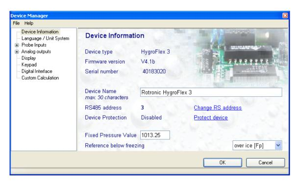
The different forms that are available within the Device Manager form are listed in a tree located on the left pane of the form. To select a form, click on it with the left mouse button.
