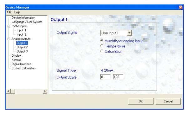
• Output Signal: select from the pull down menu (click on the arrow) to associate a probe input - or a custom calculation - with the analog output.
