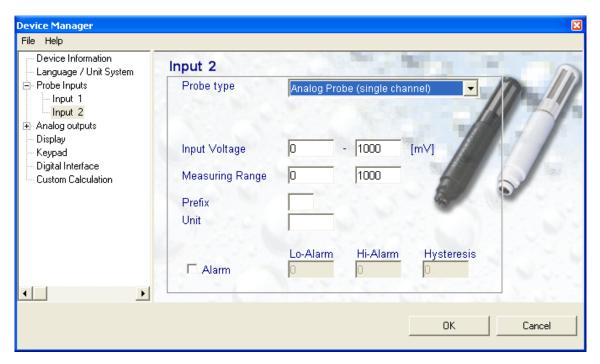
Specify the range of the input voltage (**in mV**), the measuring range of the probe, the symbol to be used on the HygroFlex display (Prefix) and the engineering unit of the parameter measured by the probe. Alarm values can be entered in the same manner as for a HygroClip probe.
