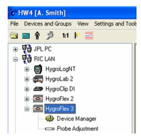
To open the Device manager form, click with the mouse on Device Manager. The Device Manager form is used to configure the HygroFlex 3 and to read instrument specific information.
