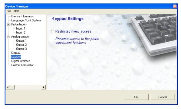
Restricted menu access: check this box to prevent tampering with the probes. Access to all probe adjustment functions from the local keypad of the HygroFlex is blocked out.
