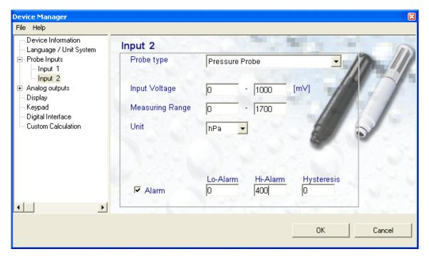
Specify the range of the input voltage (in mV), the measuring range of the probe and the engineering unit used by the probe (this may be different from the selection made under Language / Unit System). Alarm values can be entered in the same manner as for a HygroClip probe.
