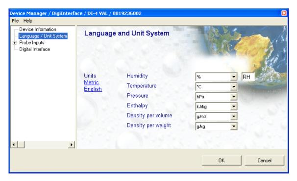
• **Units**: use the underlined links to the right of the form to globally change the unit system used by the instrument. If the unit system offers several choices such as In Hg or PSI for pressure, choose a unit by left clicking on the arrow to the right of each text box.
