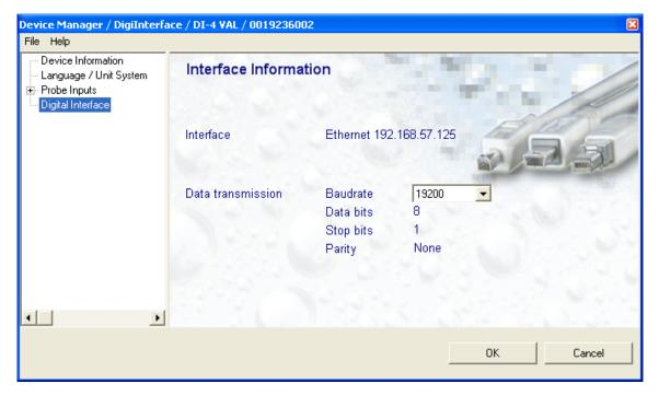
This form is used to select the RS-485 baud rate between 57600 and 19200. Other data cannot be changed from within the form. Select the Baud rate depending on which devices you plan to connect with the HygroClip DI. Devices such as the HygroFlex transmitter normally use 19200 bps.
