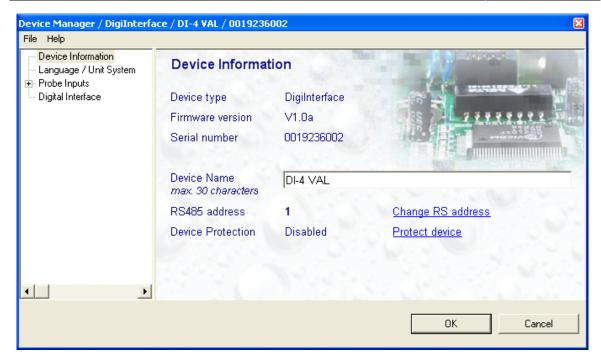
The forms that are available within the Device Manager form are listed in a tree located on the left pane of the form. To select a form, click on it with the left mouse button.
