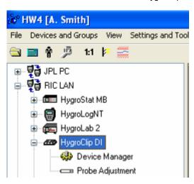
To open the Device manager form, click with the mouse on Device Manager. The Device Manager form is used to configure the HygroClip DI and to read device specific information.
