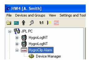
To open the Device manager form, click with the mouse on Device Manager. The Device Manager form is used to configure the HygroClip Alarm and to read device specific information.
