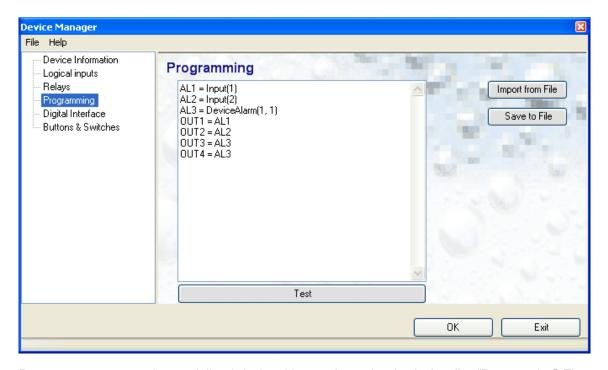
Program statements can be typed directly in the white area located under the heading "Programming". The functionality of this area is equivalent to a simple text editor.
