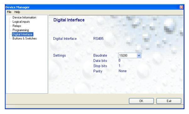
This form is used to select the RS-485 baud rate between 57600 and 19200. Other data cannot be changed from within the form. Select the Baud rate depending on which devices you plan to connect with the HCA. Devices such as the HygroFlex transmitter normally use 19200 bps.
