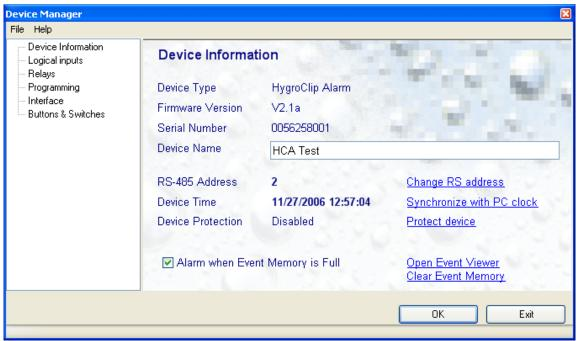
The forms that are available within the Device Manager form are listed in a tree located on the left pane of the form. To select a form, click on it with the left mouse button.
