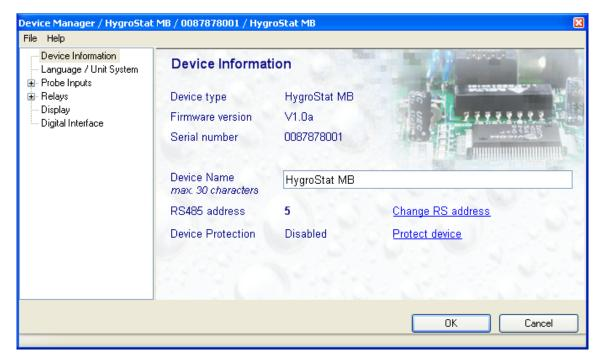
• **Device name**: this text will be displayed next to the instrument model information. As far as possible use a unique device name.
