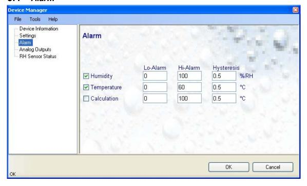
**Note**: this function applies only to the HC2 probe digital signal (digital alarm flag) and has no effect on the analog outputs.
