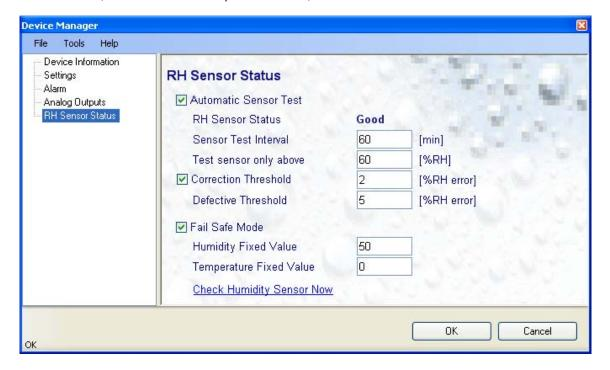
Automatic Sensor Test: place a check mark in this box to enable the automatic RH sensor test.
