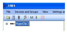
When HW4 has detected a HC2 probe, the probe appears as an icon in the left pane of the HW4 main screen. Click on the + sign to the left of the probe icon to display a list of the available functional modules.
