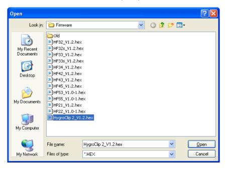
**IMPORTANT**: the probe must be powered during the entire process. Loss of power when the probe is being updated may have unexpected results and prevent future operation of the probe.
