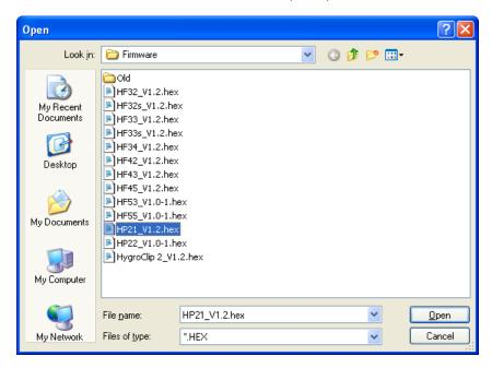
**IMPORTANT**: the HP21 must be powered during the entire process. Loss of power when the indicator is being updated may have unexpected results and prevent future operation of the HP21.
