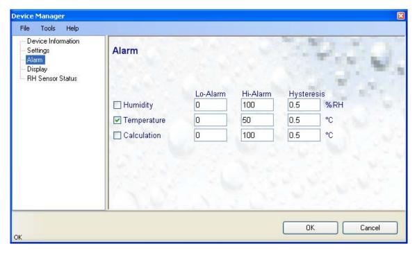
**Note**: This function applies to the HP21 display (an alarm symbol appears) and to the HP21 digital communication with a PC via service connector.
