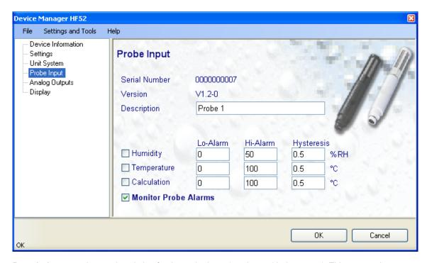
**Description:** enter here a description for the probe input (maximum 12 characters). This text can be displayed in the HW4 current Values tab.
