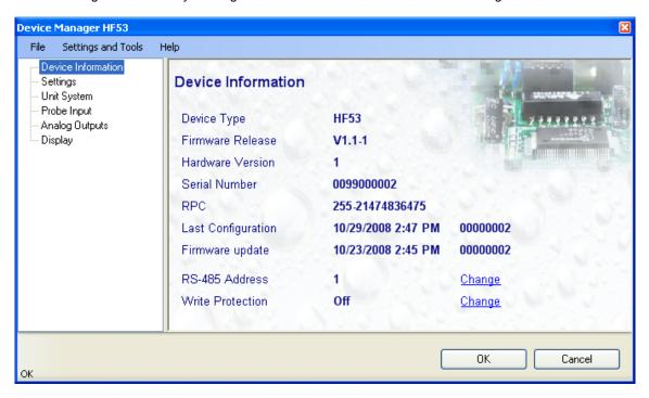
The different sub-forms that are available within the Device Manager form are listed in a tree located on the left pane of the form. The number of sub-forms depends on the HF5 model (Device Type). To select a sub-form, click on it with the left mouse button.
