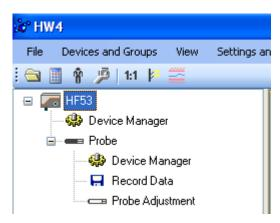
**HF53** / **HF55**: click on the + sign to the left of the probe icon to display a list of the available functional modules for the HC2 probe.
