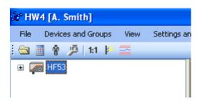
When HW4 has detected a HF5 transmitter, the HF5 appears as an icon in the left pane of the HW4 main screen. Click on the + sign to the left of the HF5 icon to display a list of the available functional modules.
