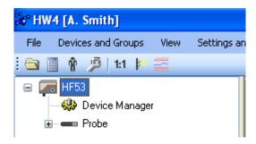
Click on the + sign to the left of the HF5 icon to display the HF5 Device Manager module.
