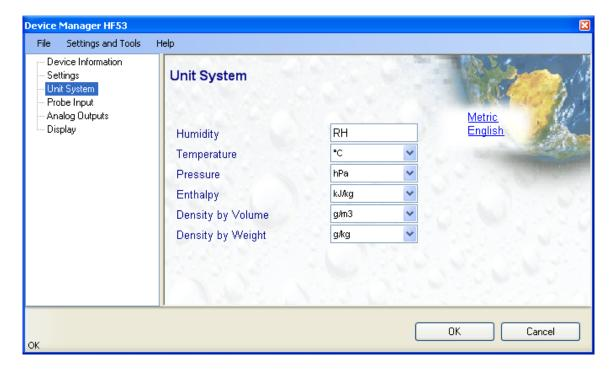
• Humidity: enter here the letters to be used after the "%" symbol used for relative humidity
