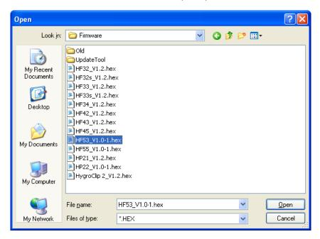
**IMPORTANT**: the HF5 must be powered during the entire process. Loss of power when the transmitter is being updated may have unexpected results and prevent future operation of the HF5.
