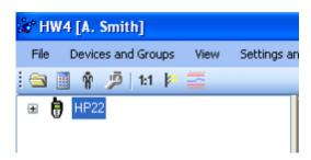
When HW4 has detected a HP22 indicator, the HP22 appears as an icon in the left pane of the HW4 main screen. Click on the + sign to the left of the HP22 icon to display a list of the available functional modules.
