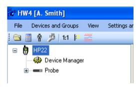
Click on the + sign to the left of the HP22 icon to display the HP22 Device Manager module as well as a probe icon.
