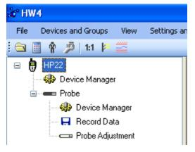
Click on the + sign to the left of the probe icon to display a list of the available functional modules for the probe.
