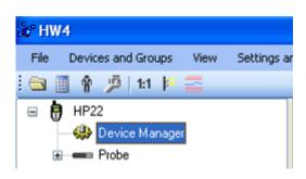
To select the Device Manager for the HP22, click on it with the left mouse button. HW4 opens the Device Manager form.
