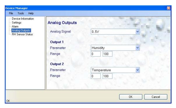
Analog signal: the type of signal for both analog outputs of the HF73 (3-wire circuit type) can be configured with HW4 as shown below:
