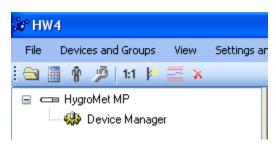
To select Device Manager, click on it with the left mouse button. HW4 opens the Device Manager form.
