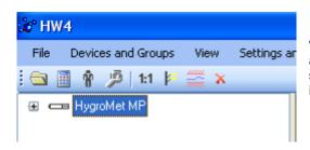
When HW4 has detected a HygroMet MP, the HygroMet appears as an icon in the left pane of the HW4 main screen. Click on the + sign to the left of the HygroMet icon to display a list of the available functional modules.
