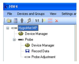
**HygroMet MP 3-wire:** click on the + sign to the left of the probe icon to display a list of the available functional modules for the HC2 probe.
