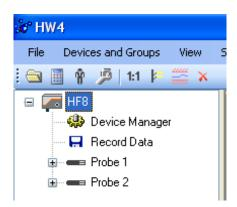
To select the Device Manager for the HF8, click on it with the left mouse button. HW4 opens the Device Manager form.
