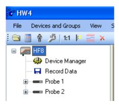
Click on the + sign to the left of the HF8 icon to display the HF8 Device Manager module, the Record Data module as well as two probe icons (one for each of the HF8 inputs). When no probe is connected, a red cross appears on top of the probe icon.
