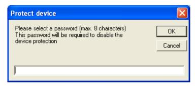
Click on the Device Manager OK button to write the new protection settings to the HFM53.
