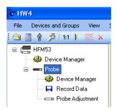
Click on the + sign to the left of the probe icon to display a list of the available functional modules for the HC2 probe.
