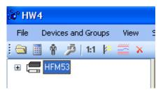
When HW4 has detected a HFM53 transmitter, the HFM53 appears as an icon in the left pane of the HW4 main screen. Click on the + sign to the left of the HFM53 icon to display a list of the available functional modules.
