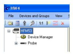
To select the Device Manager for the HFM53, click on it with the left mouse button. HW4 opens the Device Manager form.
