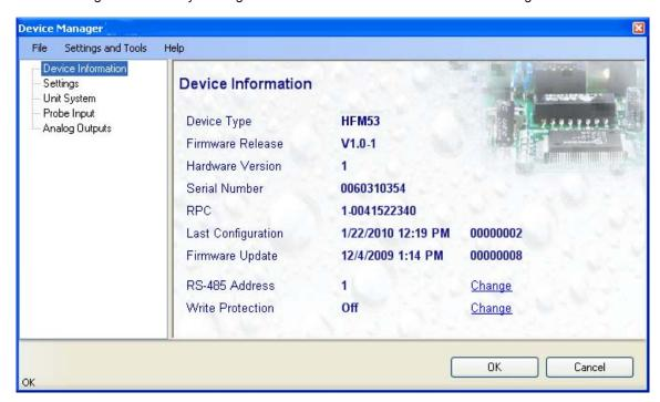
The different sub-forms that are available within the Device Manager form are listed in a tree located on the left pane of the form. To select a sub-form, click on it with the left mouse button.
