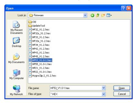
**IMPORTANT**: the HFM53 must be powered during the entire process. Loss of power when the transmitter is being updated may have unexpected results and prevent future operation of the HFM53.
