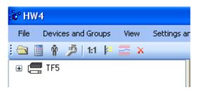
When HW4 has detected a TF5 transmitter, the TF5 appears as an icon in the left pane of the HW4 main screen. Click on the + sign to the left of the TF5 icon to display a list of the available functional modules.
