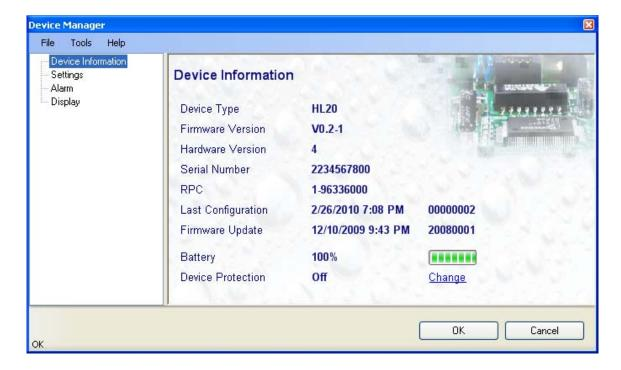
• **Device Protection**: This function is used to prevent unauthorized access to critical functions such as configuration changes, humidity and temperature adjustment, etc. Click on the underlined link next to Device Protection. HW4 opens the following form where a password can be entered (maximum 8 characters):
