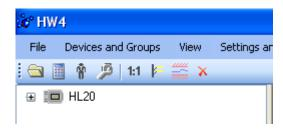
When HW4 has detected a HL20 or HL21 data logger an icon appears in the left pane of the HW4 main screen. Click on the + sign to the left of the con to display a list of the available functional modules.
