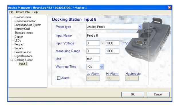
Step 2: Set the voltage source so as to generate a value as close as possible to 0.000 mV.
