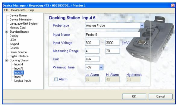
**Step 2:** Set the voltage source so as to generate a current to 4.00 mA (the nominal value of the docking station internal resistance is 150 Ohm).
