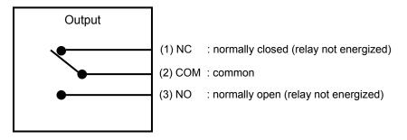
Contact Rating: 10 A at 250 VAC or 30 VDC, 12 A at 125 VAC. Please observe these ratings to avoid damaging the contacts.
