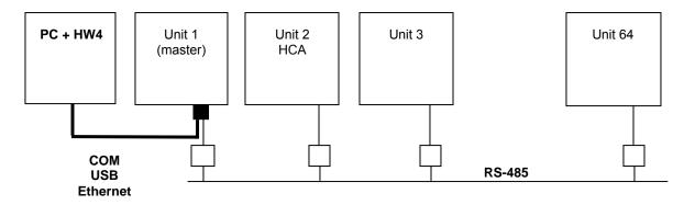
When the RS-485 network is connected to a HW4 PC, via a master, the HW4 PC takes over the task of sending data requests and instructions to the different units on the RS-485 network. Each unit remains silent unless interrogated by the PC.
