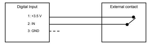
**Note**: Pin 3 (GND) is reserved for special applications and is not normally used.
