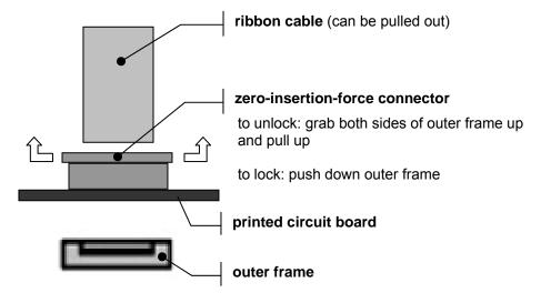
To re-attach the ribbon cable, unlock the connector (see above) and slide the cable back into the connector as indicated below. Lock the connector in place and verify the cable is firmly held in place. Each end of the ribbon cable has a contact side and a blue insulated side. When inserting the cable in the connector, position the contact side of the flat ribbon cable as indicated below.
