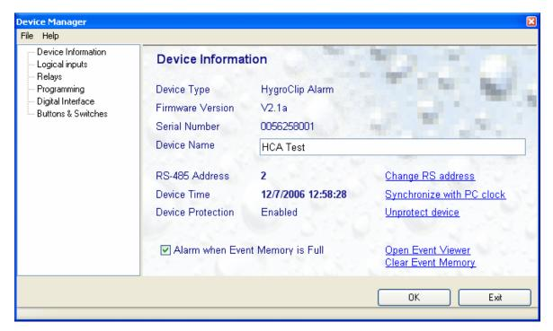
To unprotect the device and enable all functions, click on the underlined link. HW4 opens the password form:
