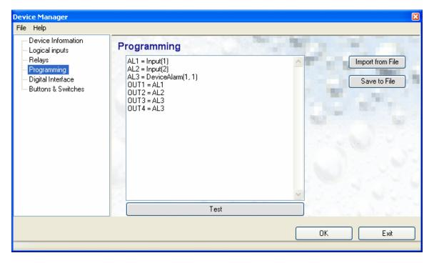
Program statements can be typed directly in the white area located under the heading "Programming". The functionality of this area is equivalent to a simple text editor (see screen shot below). See <a href="Programming the HCA">Programming the HCA</a>
