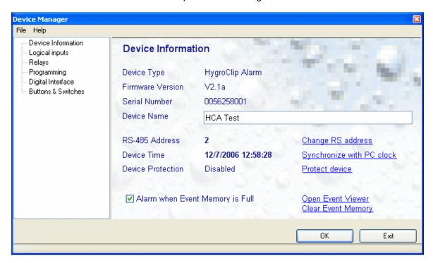
To protect the device, click on the underlined link. HW4 opens the following form where a password can be entered (maximum 8 characters):
