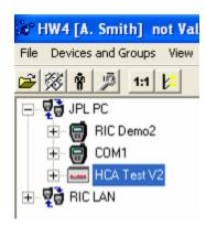
6) In the HW4 device tree, click on the + sign to the left of the HCA to display the Device Manager. Click on Device Manager:
