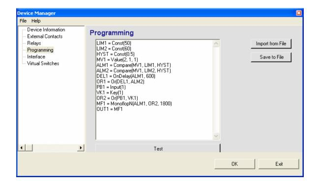
All programming statements can be typed directly in the programming field (same as with a text editor). The syntax can be checked by clicking on the "Test" button. Any line with a syntax error is automatically highlighted.
