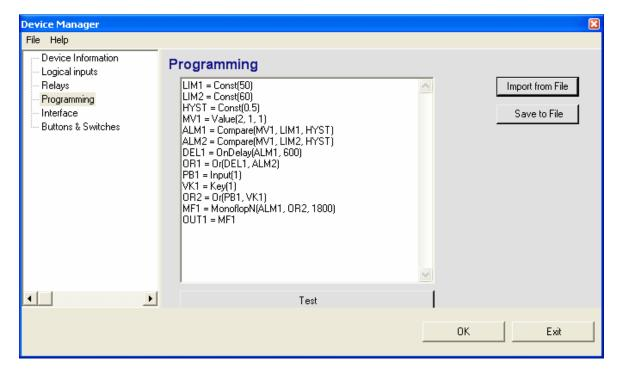
Program statements can be typed directly in the white area located under the heading "Programming". The functionality of this area is equivalent to a simple text editor (see screen shot below).
