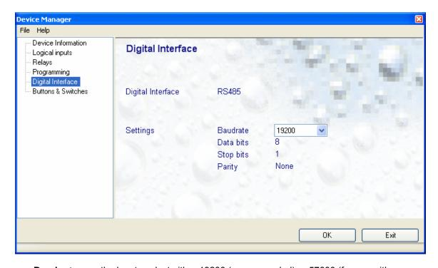
• Baud rate: use the box to select either 19200 (recommended) or 57600 (for use with HygroLog NT and HygroClip Interface only)
