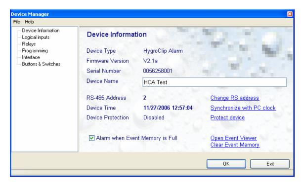
• **Device name**: this text will be displayed by HW4 next to the device icon. If possible use a unique device name.
