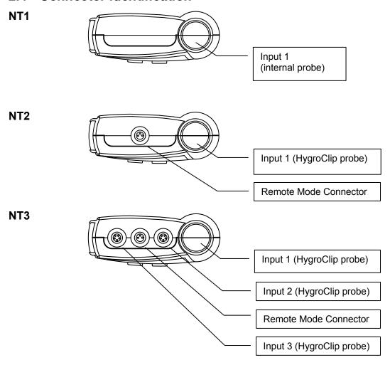
Note: an adapter cable is required to connect a probe to input 2 or 3 of the HygroLog NT3. Use cable MOK-02-B5 (or similar) for probes with a 5-pin DAT-05 connector. Use cable T7-03-B5 (or similar) for probes with a 7-pin T7 connector.
