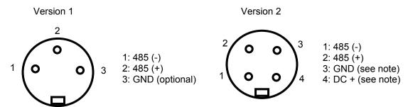
Note: use pins 3 and 4 to power multi-dropped instruments with a single external 12 VDC power supply with adequate mA rating. Pin 4 and the 12VDC power jack of the docking station are not connected.
