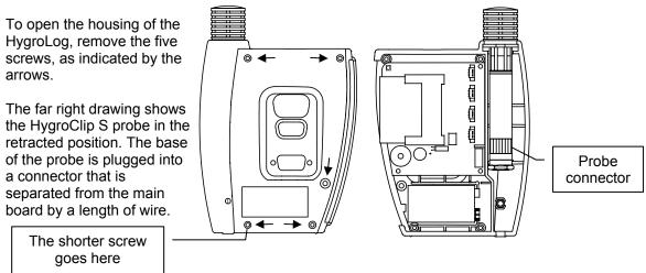
To extend the probe, lift the HygroClip S probe from its position and remove the slotted cap from the HygroLog. To extend the probe, place on the probe the ring supplied with the HygroLog.
