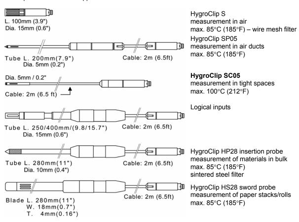
Note: the above probes have a 5-pin DAT-05 connector. An extension cable such as the MOK-02-DAT05 can be used to connect any of the above probes to input 1 of the HygroLog NT2 / NT3 (this input is normally used for an internal HygroClip S probe). An adapter cable such as the MOK-02-B5 is required to connect any of the above probes to inputs 2 and 3 the HygroLog NT3 or to inputs 4 to 7 of the docking station (see Accessories).
