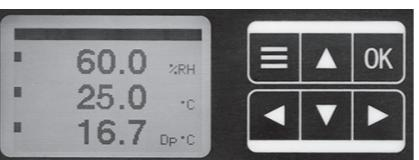
Note: Unauthorized use of the menu can be prevented by disabling the setting "Display Menu" (setting with HW4 software).
