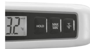
**HOLD:** The HOLD button freezes the display, and switches on the backlighting of the display.
