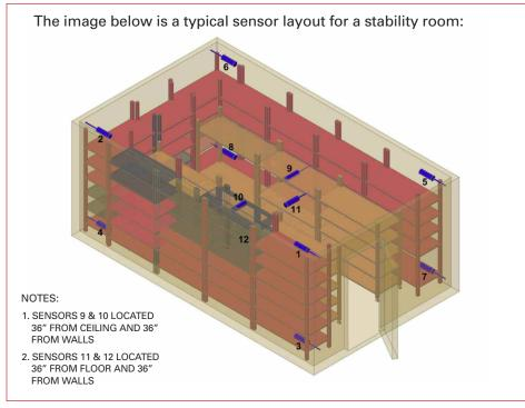
Sensors should be placed in typically known reduced air flow locations. This diagram may not be representative of actual chamber shelves, racks, or cages used to store samples. The table below describes actual sensor placement locations.
