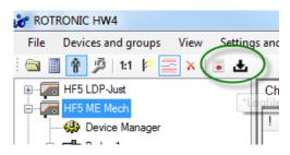
Buttons for bulk download of files and direct generation of PDF report or direct creation of PDF report based on existing log files on the PC.
